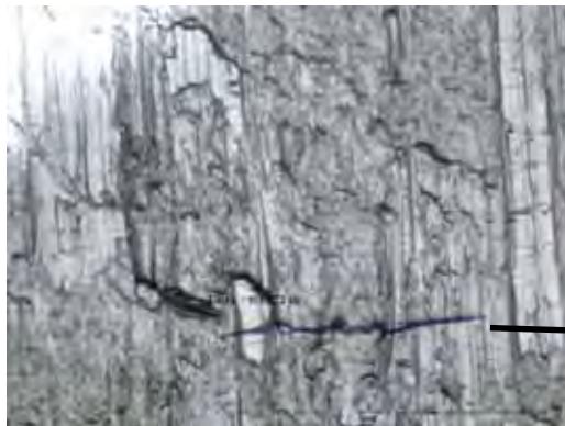
Crack on front side at 43,000 cycles
