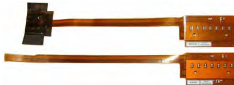
MWM-Array FA43 Sensor
