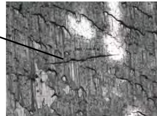
Crack on back side at 43,000 cycles
