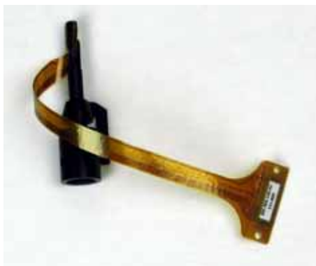
Mandrel Assembly with interchangeable MWM-Arrays
